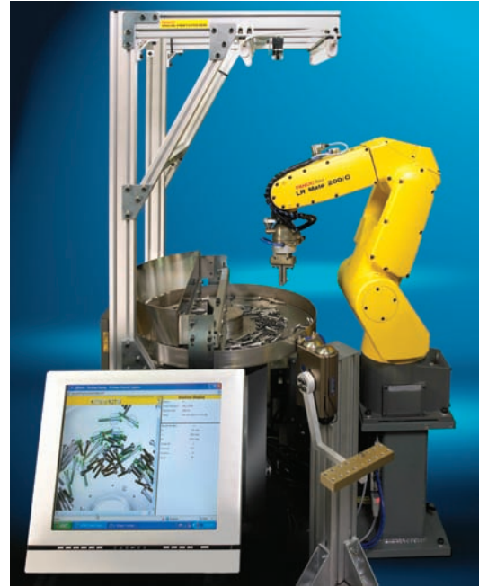
LR Mate 200iC picks & sorts multiple style parts through flexible feeder using built-in iRVision and available Aux. Axis option!
